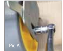
M12 nyloc nut torque to 80Nm. M12 standard washer. Special thin spacer washer on top of swivel bearing of castor M12X60 10.9 bolt
