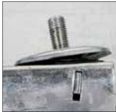
Mounting plate distortion as a result of a single significant impact or multiple lower level impacts. Even if the rest of the castor is in good condition, it must be replaced.
